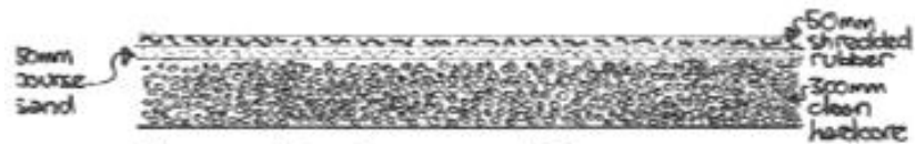
Cross-section of manege 1:20
